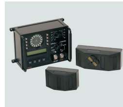
LAWAREC BRICK Laser/Radar Warning Receiver
