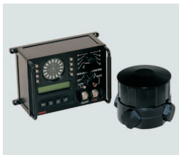
LAWAREC LW5-8D-4R Laser/Radar Warning Receiver
